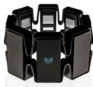
SIPL students have started to work with the Myo Armband for **real time EMG signal acquisition**. An EMG signal records electrical activity produced by skeletal muscles.
