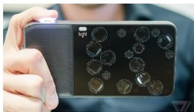
Light L16 is a **revolutionary point-and-shoot camera** that packs 16 cameras that simultaneously expose photos at different focal lengths. The resulting images are combined into high-resolution, 52-megapixel photos.
