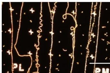
A team from *SIPL* has cooperated with Prof. Yuval Yaish to create a breakthrough technology that could help **replace silicon chips with molecular electronics based on carbon nanotubes** as the building block of electronics. Our team dealt with the task of recognizing nanotube lines in noisy images. [A paper describing this work](#) was published in Nature Communications. More information can be found [here](#).
