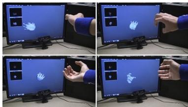
DeepHand is an algorithm from researchers at the University of Purdue that uses deep learning to **estimate the 3D pose of a hand** using depth data. [A paper describing this work](#) was presented in CVPR 2016. A demo video can be found [here](#).
