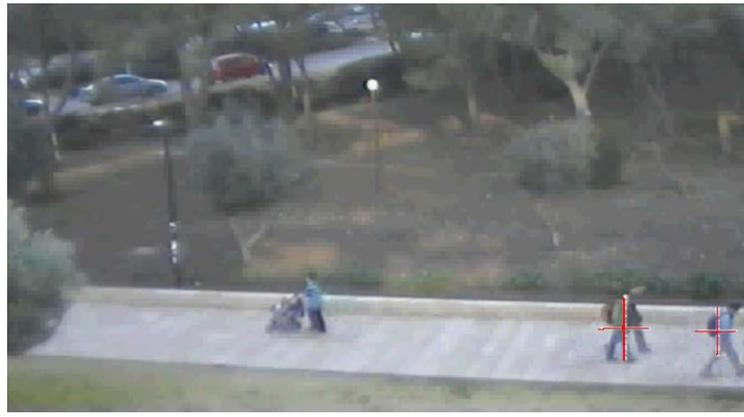
**Figure 4:** Imperfect pedestrian tracking example. The left pedestrian is detected together with the stroller and is discarded due to non-legitimate height-width ratio.
