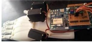
The work of two *SIPL* students who developed a **3D printed robotic prosthesis hand** was described in the January 2017 issue of the IEEE Signal Processing Magazine. Controlling the prosthesis is based on an EMG signal (electrical activity produced by skeletal muscles).
