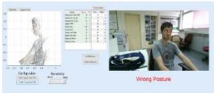
**Project in the spotlight:** Two *SIPL* students have developed a **system that analyzes the user's posture**. A Kinect depth camera is used to detect wrong sitting positions such as leaning backward/forward, leaning sideways, titled-down head, body rotation etc. In a lightweight background application, posture parameters are constantly monitored. When a wrong sitting posture is detected for a prolonged time, the system alerts the user and guides him back to the right posture.
