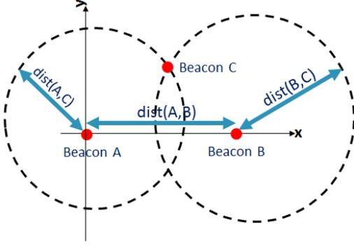
Figure 4: Beacons Positioning through distances measurements and circles intersection
