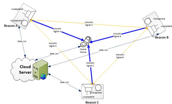
Figure 1: proposed Acoustic Positioning System Configuration
