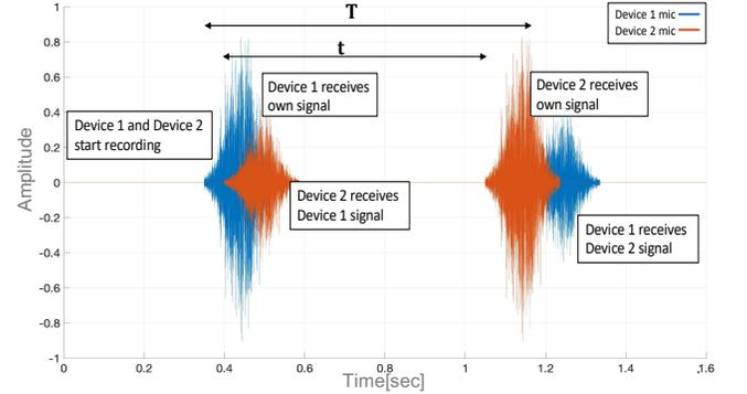
Figure 2: Active Devices Distance Measurement
