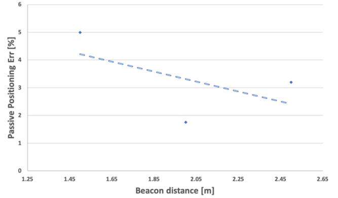
Figure 10: Passive Device positioning error with equilateral triangle Beacons setup
