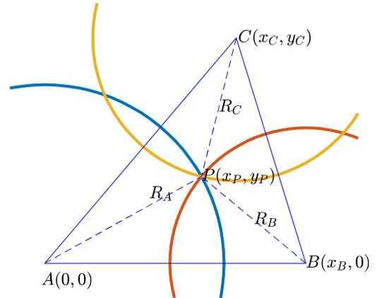
Figure 5 – Geometric layout of the system elements - beacons A, B, C and a mobile device P at the intersection point of the three circles.
