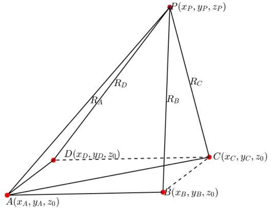
Figure 6 – Geometric layout of the system elements - beacons  $A, B, C, D$  and a mobile device  $P$ .
