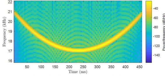
Figure 2 - Spectrogram of a parabolic chirp
