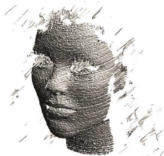
Figure 4: Raw depth image of a human face reconstructed using the proposed fixed-point algorithm
