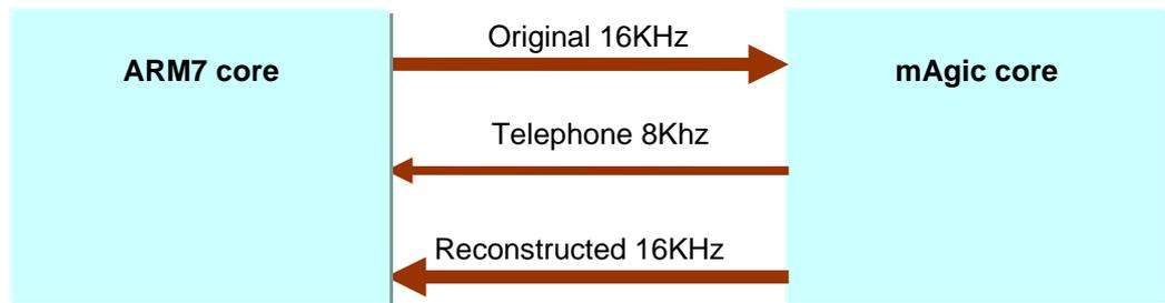
Since it is impossible to configure different output channels of the ADDA to operate at different frequencies, we operate all channels at 16 KHz frequency. The lowband signal, intended for the telephone channel, is upsampled prior to sending it to ARM (still, it lacks the 4 KHz to 8 KHz frequency components).
