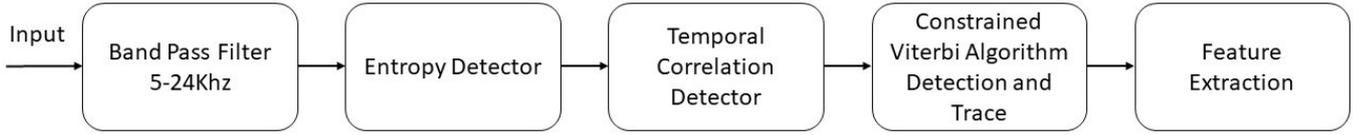
Fig. 2: A block diagram for the operation of ECV
