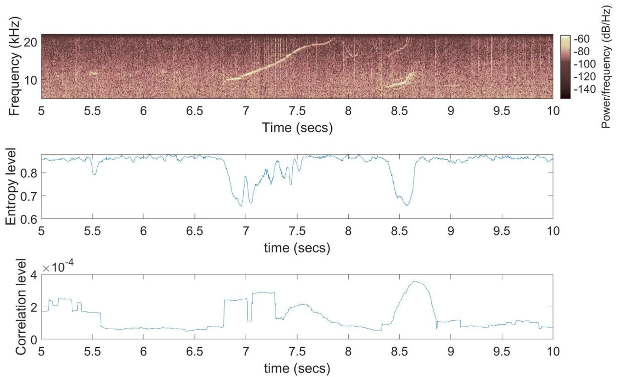
(a) The upper panel shows a spectrogram containing two dolphin whistles. The middle panel shows an entropy detector and we observe a decrease of the entropy level where a whistle exists. The lower panel shows the output of the temporal correlator, and an increase is observed where whistles are located. Recording was collected off the coast of Ashdod, Israel in May 2018.
