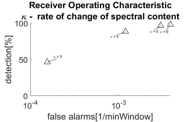
(d) ROC for the Viterbi Algorithm detector. For SNR=0 dB, good trade off between detection and false alarm rates is obtained for  $\kappa = 4$ .
