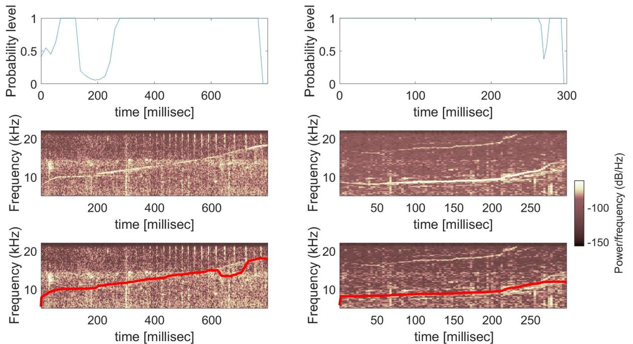
(b) Illustration of the constrained Viterbi module. The module first calculates the path probability, and then traces the whistles' contours. Notice that the algorithm will always find a path and is susceptible to deviate due to strong noise signals
