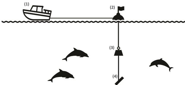
Fig. 1: An illustration of the recording technique used to record dolphin whistles. The surveying vessel (1) moves in order to cover large geographical area. The hydrophone (4) is connected to the vessel using a cable which is attached in two connection points: to a buoy (2) and a weight (3). The buoy keeps the cable floating behind the vessel, and the weight is attached close to the hydrophone.
