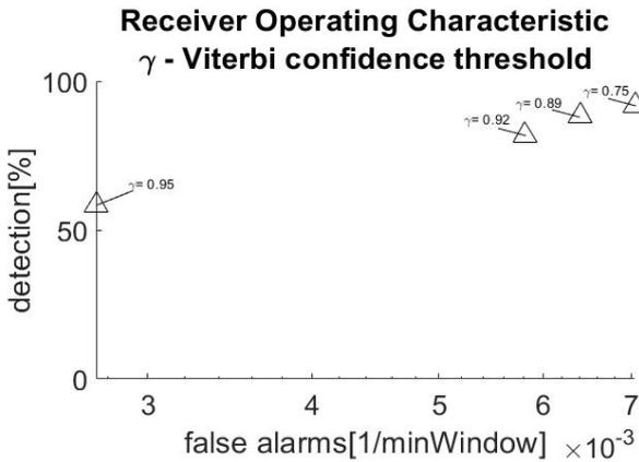
(c) ROC for the Viterbi Algorithm module noise threshold. For SNR=0 dB, good trade off between detection and false alarm rates is obtained for  $\gamma = 0.92$ .
