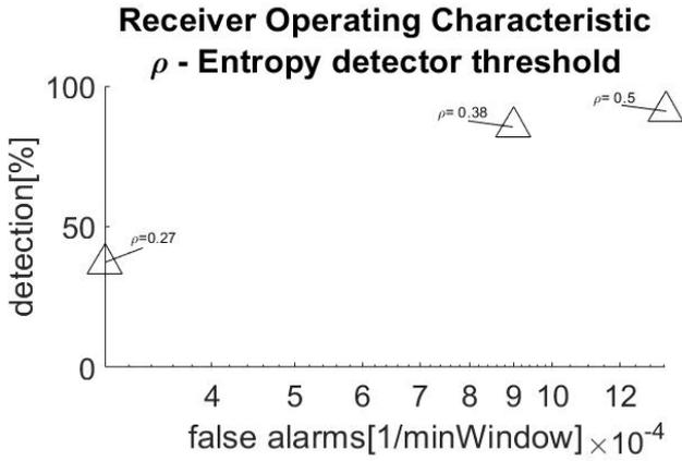
(a) ROC for the Entropy detector. For SNR=0 dB, results show a good trade off between detection and false alarm rates for threshold  $\rho = 0.38$ .
