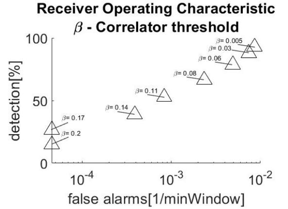
(b) ROC for the Correlation detector. For SNR=0 dB, good trade off between detection and false alarm rates is obtained for  $\beta = 0.06$ .
